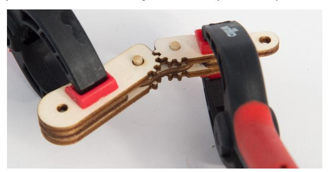
Fit the hand into place as shown. The wrist pin is glued at each end but free to move in the middle so that the hand can move. Fit the shoulder pin into place.
